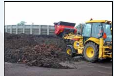
Mixing sludge and bark
