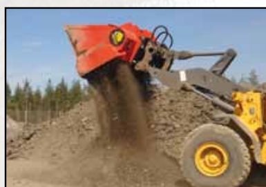
Aerating contaminated soil compost
