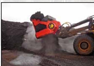
Aerating sludge compost
