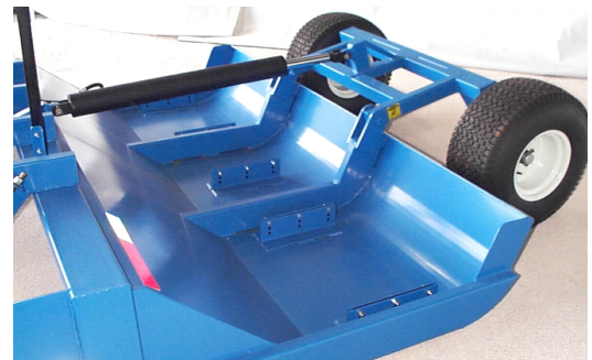
Multiple, adjustable and replaceable skes in the pan reduce side hill slippage on uneven terrain. The high, radiused lip on the rear of the pan "ramps" the drag up onto the snow when backing up. The hydraulic rear wheel assembly with high flotation tires provides plenty of height when needed.
