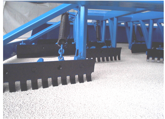
The standard serrated cutting blades are very effective in those hard icy trail conditions. Blade support struts have been rotated 45 degrees to promote the free flow of snow through the drag.
