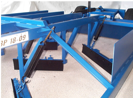
The heat treated cutting blades are adjustable and have a unique adjustment stop that keeps the blade in place when set. Spring tripping cutting blades are a must for early season grooming.
