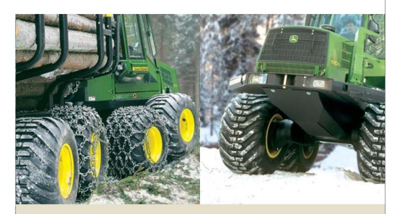
The patented balanced bogie distributes the weight evenly between all wheels. This reduces the ground impact and ensures a gentle ride even when the forwarder is fully loaded.
