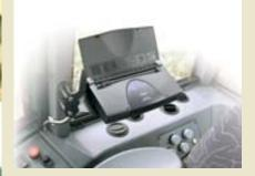
The software features a versatile fault diagnostics function and the system issues reminders of scheduled maintenance services. The reports produced by the Timbermatic 700 can also be printed out using an A4 size colour printer.
