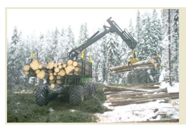
The strongly built long-reaching booms are positioned at an appropriate distance almost parallel to the operator's field of vision. This allows for smooth and natural controlling of movements. Optional equipment include hydraulic dampening of the slew and lifting motions and an ASF function for the boom of the 810D, which adjusts the position of the boom and holds the grapple still above the load while the machine is turning.
