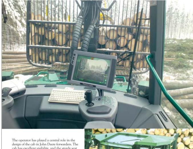
The operator has played a central role in the design of the cab in John Deere forwarders. The cab has excellent visibility, and the sturdy seat and ergonomically designed controls ensure that the operator does not get tired. The comfort of the working environment is further improved by the optional sun blinds, the efficient air conditioning and heating system and the cabin filter, which keeps the interior air of the cab fresh and clean.
