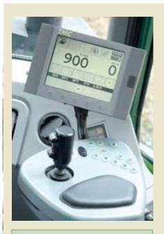
The Timbermatic 700 and the TMC improve overall productivity and allow for easy use of the latest monitoring tools, such as the boom scale and the reverse camera. The sensors and software of the optional boom scale measure the weight of the load and the logs. This allows for efficient use of the load space: the loads remain a suitable size and forwarding is safe and fast. The self-learning calibration function of the scales increases the reliability of the system.
